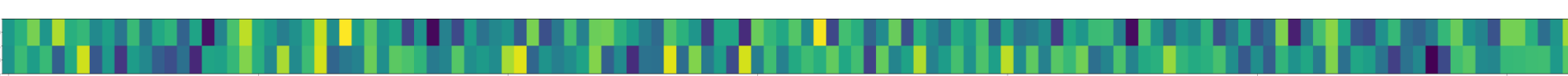
Fig. 3. A CPSK input vector of length 128, as an "image" input to the CNN model. The first row consists of the In-phase (I) components, the second row of the Quadrature-phase (Q) components.
